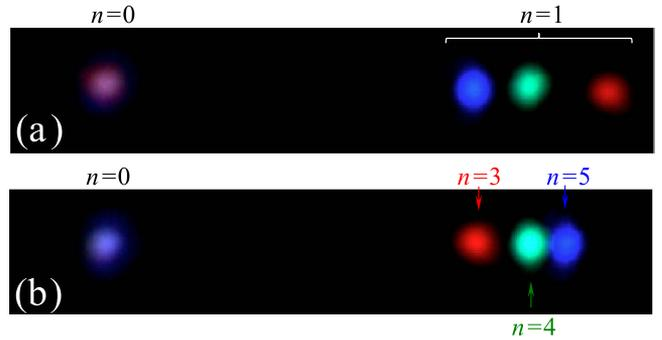
Fig. 3. Superposition of the diffraction patterns for wavelengths of 633, 514, and 454 nm for (a) blazed grating operating in the first diffraction order and (b) blazed grating operating in higher diffraction orders. For the sake of comparison, the grating in (a) has a period four times shorter compared to (b) in order to achieve the same diffraction angle for 514 nm.
