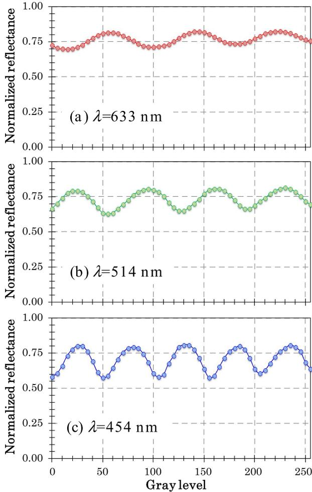
Fig. 1. Normalized reflectance as a function of the addressed gray level for wavelengths of (a) 633 nm, (b) 514 nm, and (c) 454 nm. Input polarization is selected parallel to the LC director.
