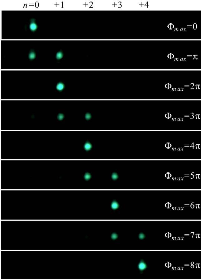
Fig. 2. Diffraction pattern as a function of the maximum phase shift  $\Phi_{\max}$  of a blazed grating when it is growing from zero to  $8\pi$  radians. Light intensity is progressively transferred from zero to fourth diffraction order.
